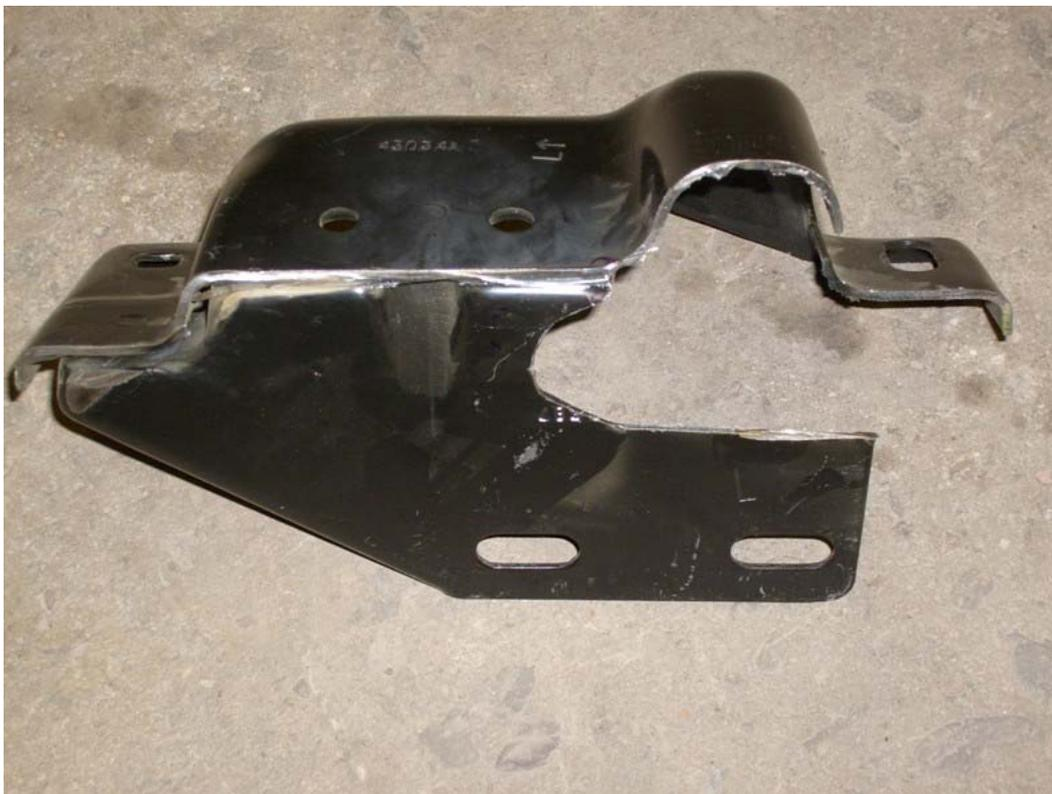
Figure 9: Bumper Mounting Bracket (Driver Side)
