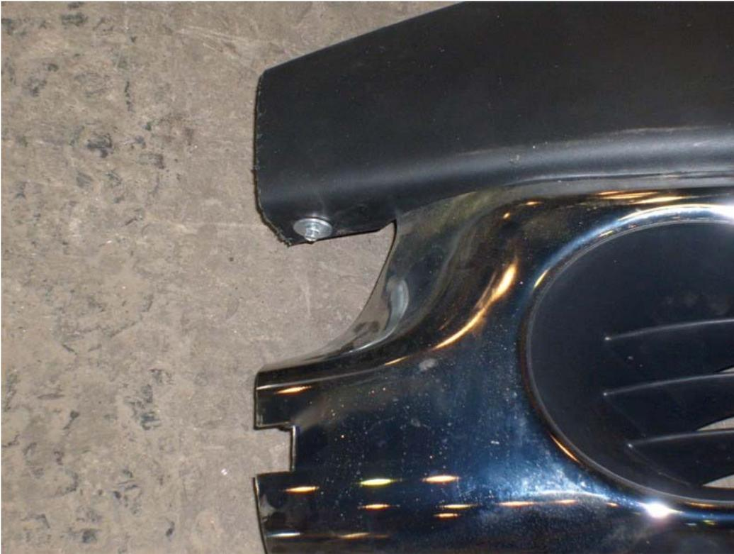
Figure 12: Bumper Modification (Drivers Side Corner)
