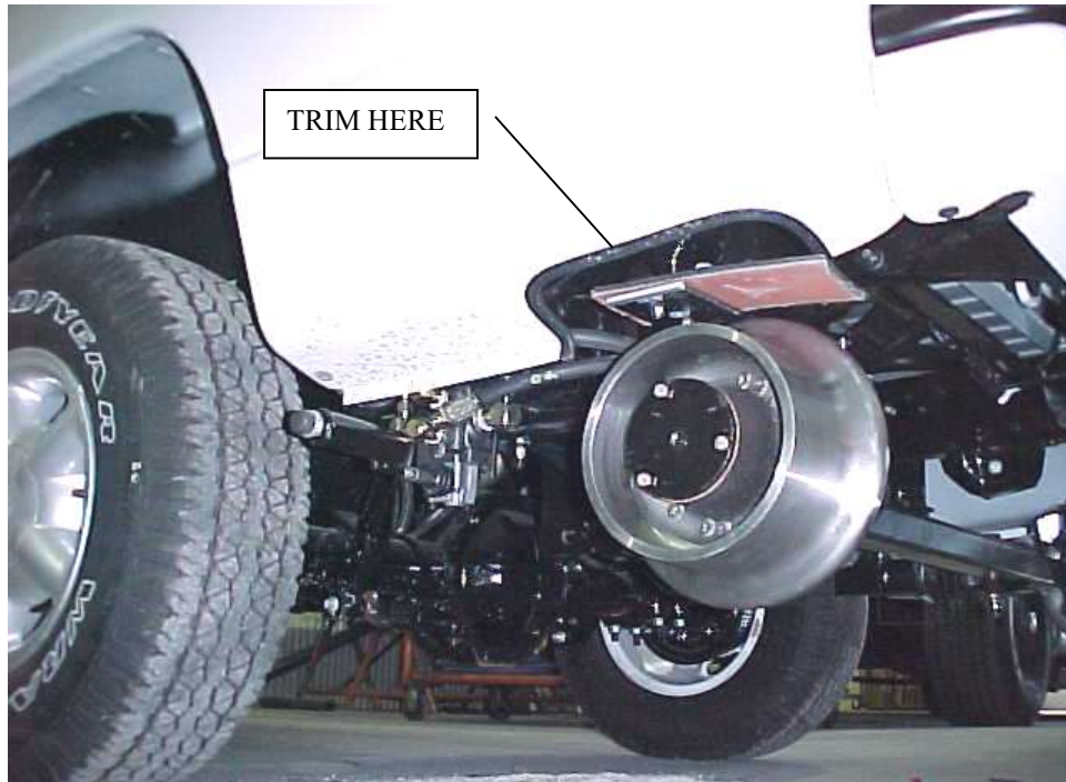
FIGURE 3-6: DAKOTA REAR FENDER MODIFICATION
