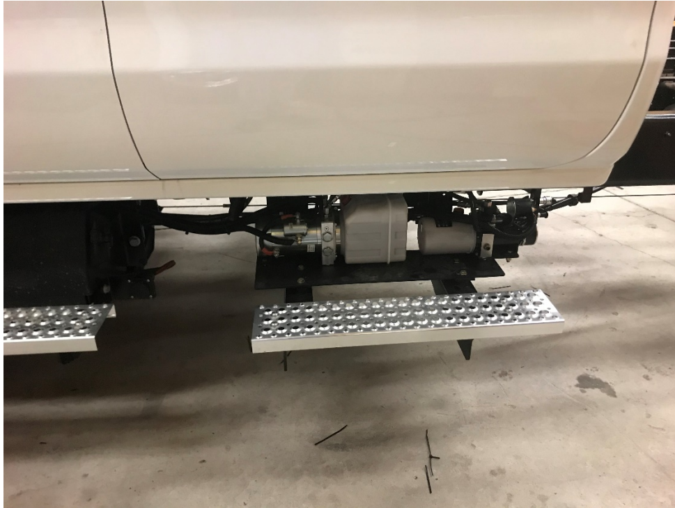
Photo 1: Hydraulic Pump and Brake Pump Installed
