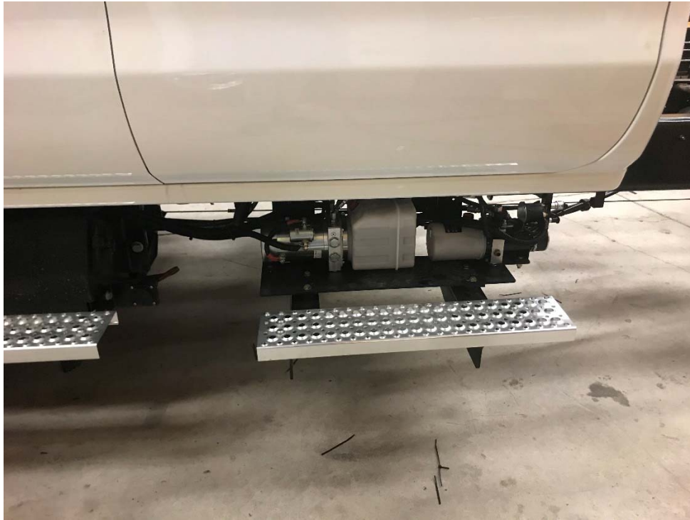
Photo 2: Hydraulic Pump and Brake Pump Installed
