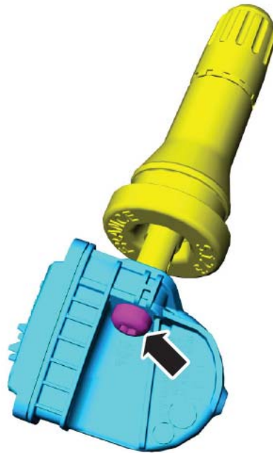
Figure 4 TORQUE TO 12 IN-LBS
