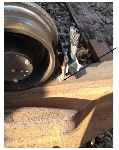
Photo on the left shows the Shunt/Sweep set too extreme. This is not acceptable and should be avoided.
