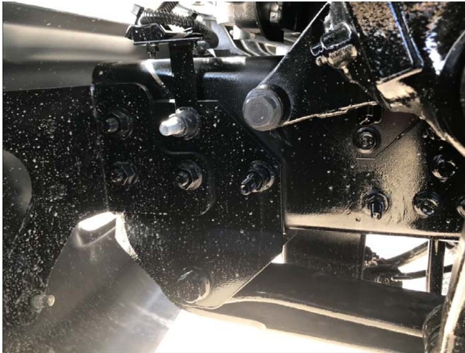
Figure 1: Non Huck Bolts for Bumper Bracket and Leaf Spring Bolt
