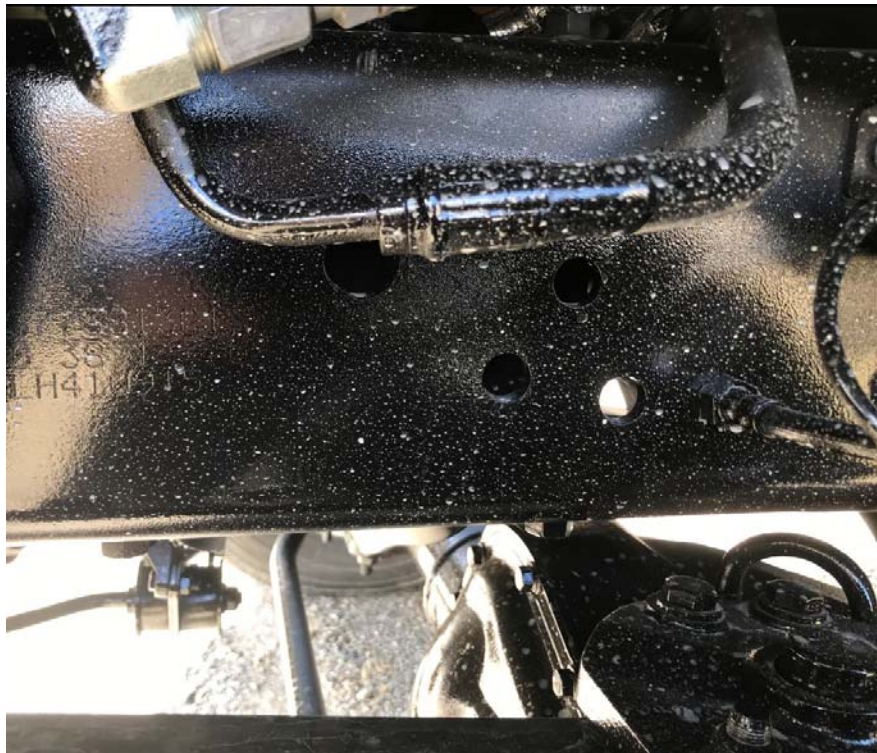
Figure 2: Snow Plow Prep Holes in Frame
