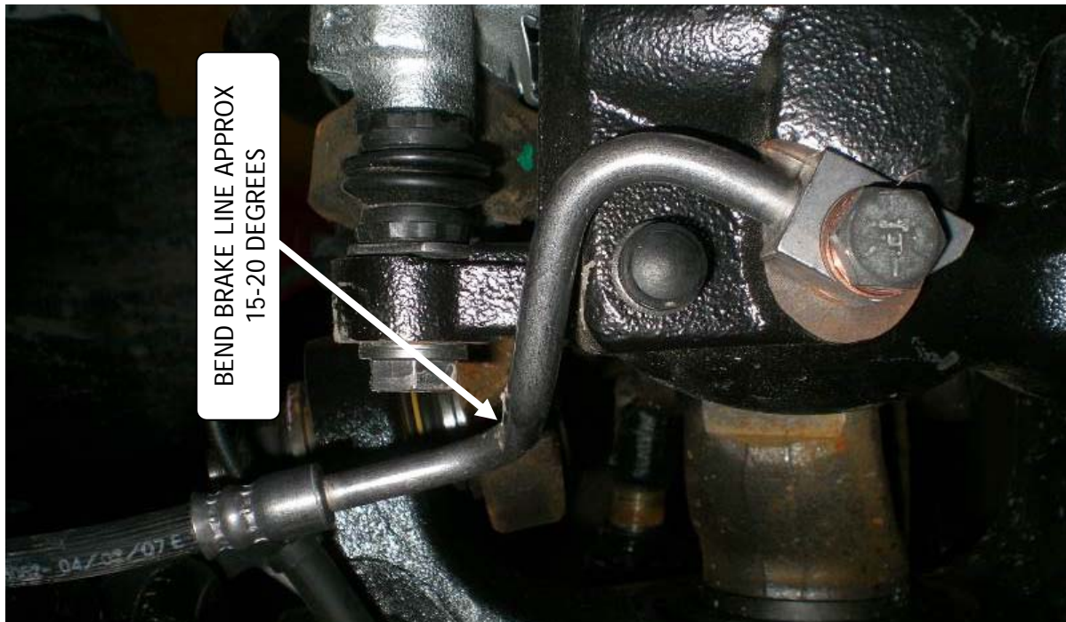
Figure 1 BRAKE LINE BENT AT APPROX. 15-20 DEGREES
