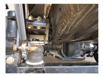
2. THE PASSENGER'S SIDE PIVOT BOX ALSO COMES IN CONTACT WITH THE TANK CRADLE. **G&B Specialties Inc.** 535 West 3rd Street, Berwick, PA, USA Tel: 1-570-752-5901 Fax: (570) 752-6397
