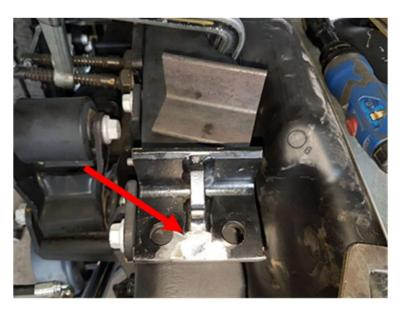
LOWER PORTION OF THE BRACKET NEEDS TO BE TRIMMED, AND GUSSET REMOVED.
