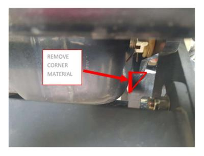
REMOVE APPROXIMATELY 3/4" X 3/4" FROM THE CORNER OF THE LOCK LATCH. THIS IS
