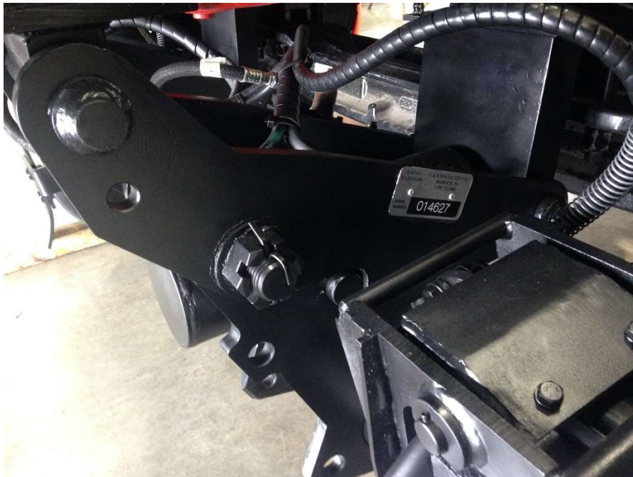
PHOTO 1: GENERAL LOCATION OF FRONT RAIL GEAR SERIAL NUMBER
