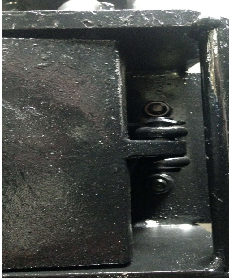
PHOTO 6: CLEVIS PIN IN BRAKE ACTUATOR ARM
