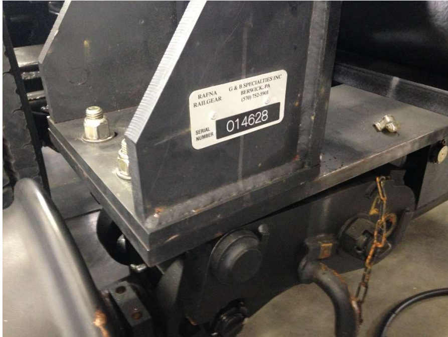
PHOTO 2: GENERAL LOCATION OF REAR RAIL GEAR SERIAL NUMBER
