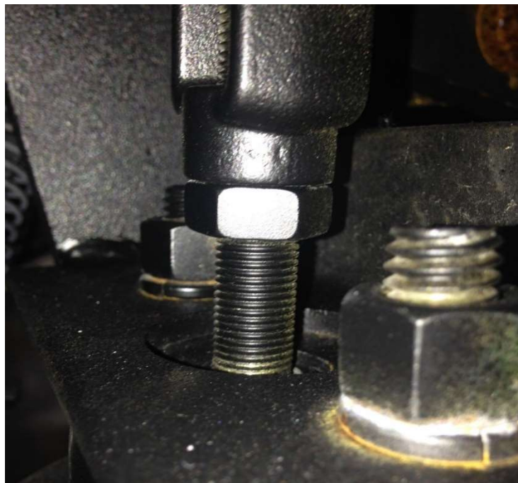
PHOTO 5: CLEVIS AND JAM NUT
