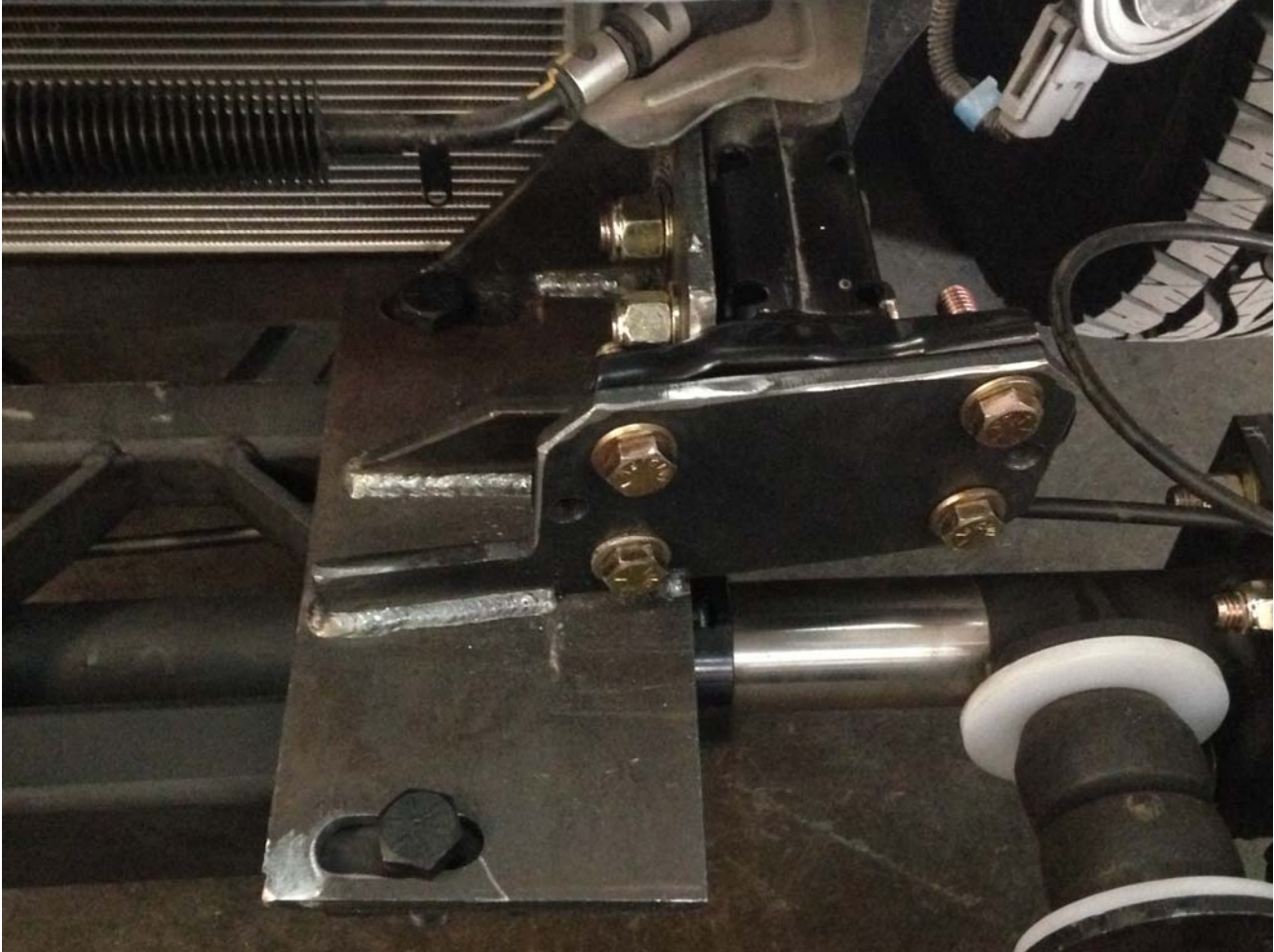
Photo 1: Horn Mounting Plate Welded to Mounting Bracket
