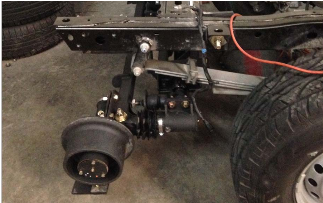
Photo 2: Square Washer Installed
