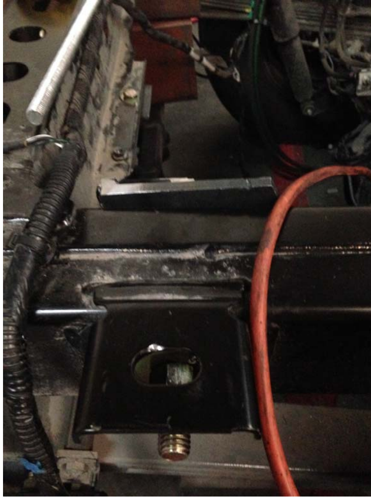
Photo 1: Bed Mount and Bolt Installed
