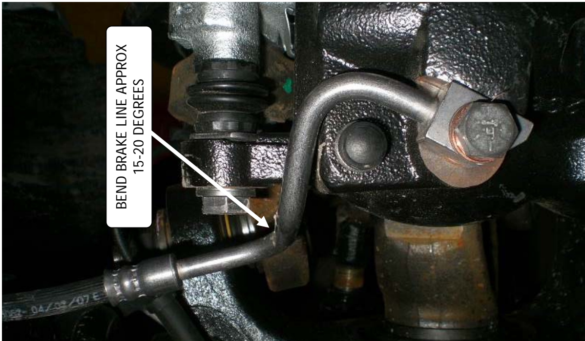
Figure 1 BRAKE LINE BENT AT APPROX. 15-20 DEGREES
