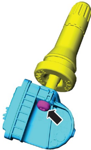
Figure 4 TORQUE TO 12 IN-LBS
