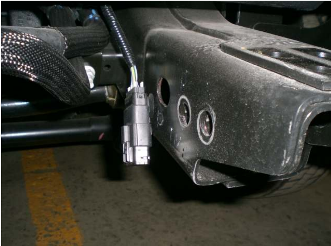
Figure 2: Connector Location and 7/8" Bolt Hole
