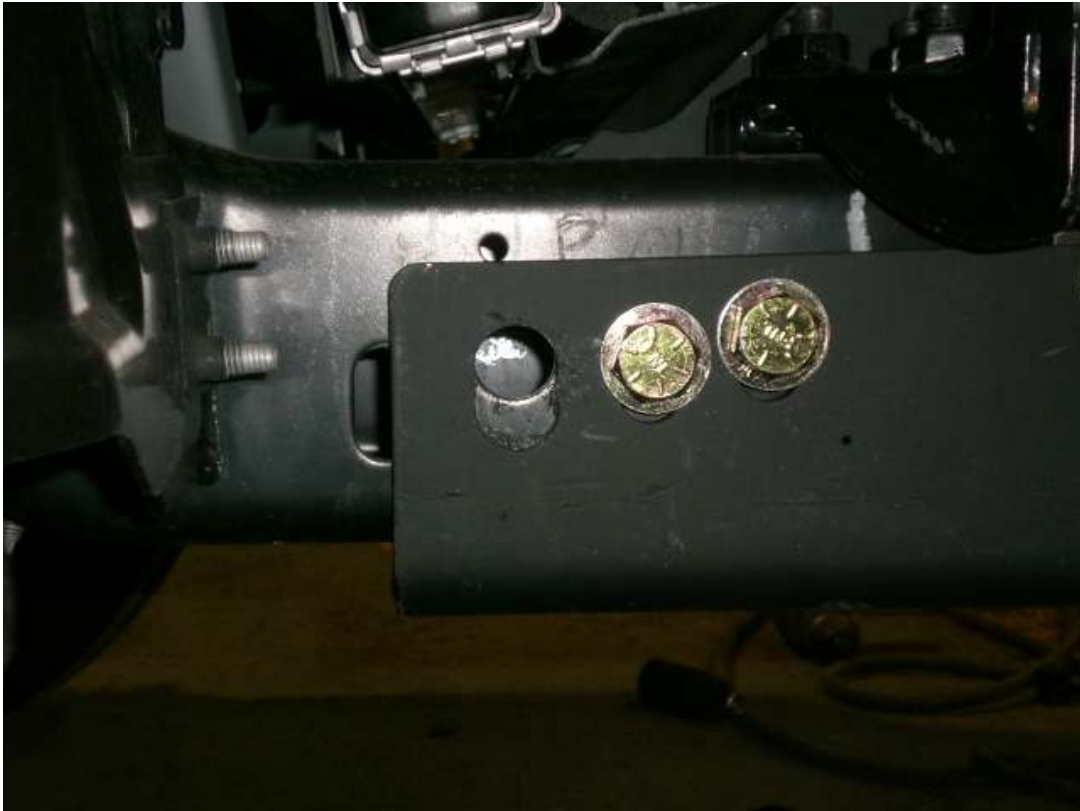
Figure 4: Through Hole for 7/8" Bolt
