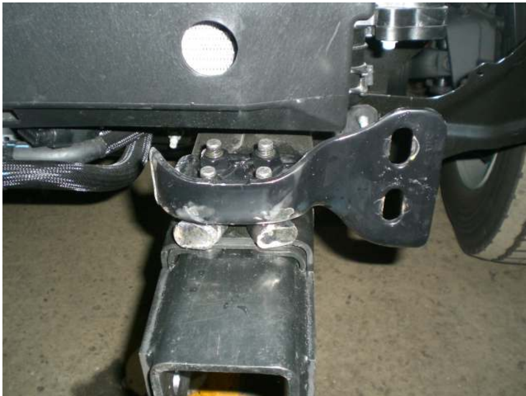
Figure 1: Modification of Tow Hook (Driver's side shown)
