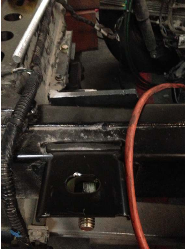
Photo 1: Bed Mount and Bolt Installed
