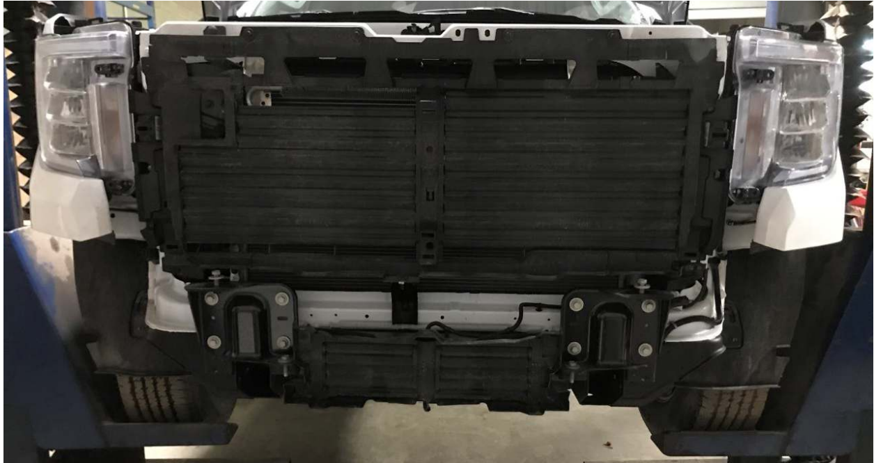
Bumper, Brackets etc. Removed From Truck
