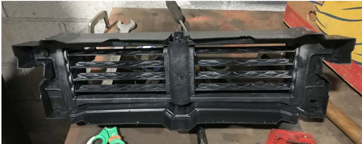
Louvers and Housing Removed From Truck
