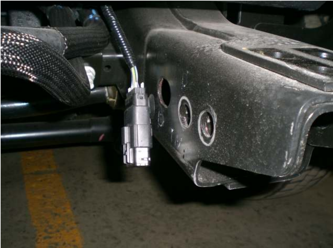
Figure 2: Connector Location and 7/8" Bolt Hole
