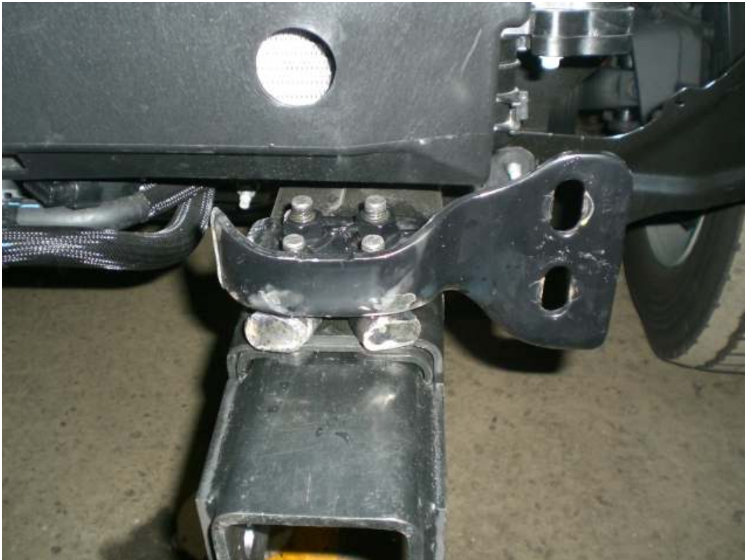
Figure 1: Modification of Tow Hook (Driver's side shown)
