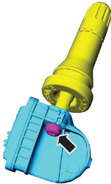
Figure 4 TORQUE TO 12 IN-LBS
