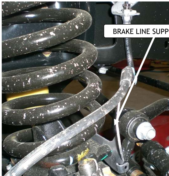
Figure 2 Support Bracket - before bending
