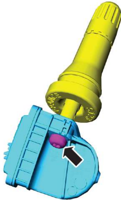
Figure 4 TORQUE TO 12 IN-LBS
