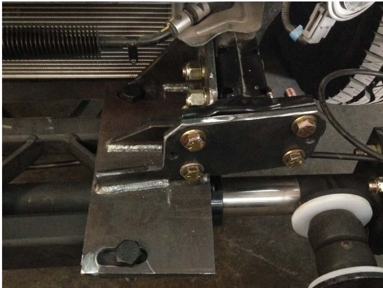
Photo 1: Horn Mounting Plate Welded to Mounting Bracket
